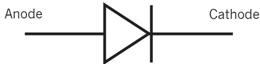
*Most diodes have a dot or a bar on them that shows which lead is the cathode:*
