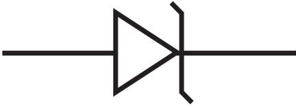
In the forward direction or when only small voltages are applied, a Zener diode works just as does a general-purpose diode. However, the Zener diode is designed so that the reverse breakdown takes place at a precise voltage, which can be as small as 1.8
