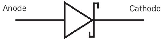
This also makes the Schottky diode capable of operating as a fast switch –the switching time for the 1N6263 Schottky diodes in your kit is about 100 picoseconds – fast enough to keep up
