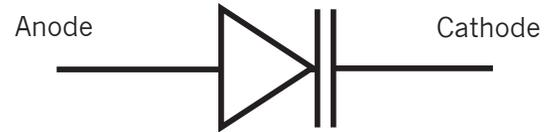
The operating principle of a varicap diode can be illustrated through the check valve analogy. When a diode is reverse-biased (as in the second part of the check valve picture), initially electrons are pressed up against the
